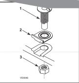
2. Hand tighten the 2 plastic drain fittings (1) using the gaskets (2) and nuts (3) as shown. Close the door.
